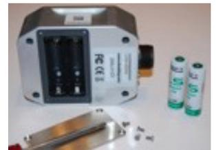
**Note:** All ShockLog units are rated to IP67. The battery compartment is isolated from the main body of the ShockLog unit and a poor fitting of the battery cover will not dramatically affect the IP rating of the main unit. However, if there is water ingress into the battery compartment, the batteries are likely to short and cause corrosion of the battery terminals. If this corrosion occurs, the ShockLog will not function correctly, and the unit will need to be returned to SpotSee for repair.
