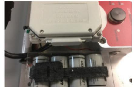
Prior to use, the satellite module will show OFF on the end of the module.
