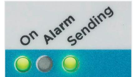
**Alarm Triggered** - When SpotBot experiences an impact above the “Alarm Threshold,” the “Alarm” (red) as well as the “On” and “Sending” (green) lights will flash at different intervals. The lights continue to flash as the SpotBot unit sends the alarm data to the SpotSee Cloud.
