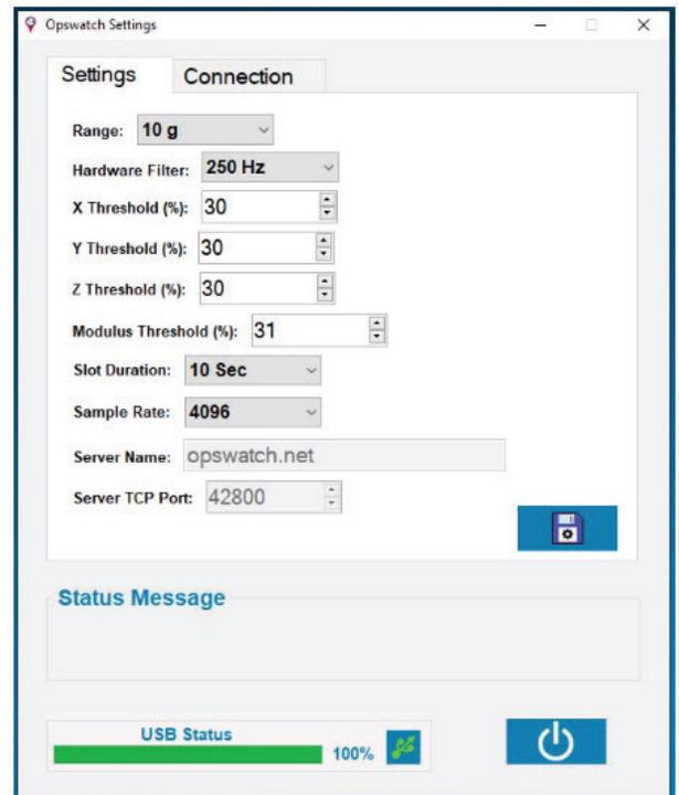
The user will set the range, filter, impact alarm level, sample period (slot duration) and sampling rate. The settings are explained below:
