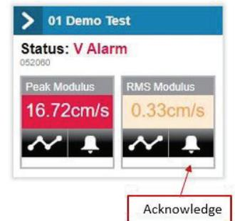
To clear an RMS Critical Alarm, click on the Graph icon to open the RMS graph page and then click Reset to clear the critical alarms.
