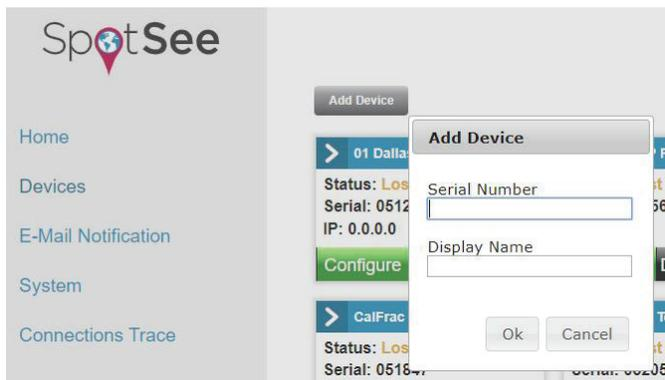
Click the Add Device button. A window will open to enter the OpsWatch serial number and display name. The display name should be something meaningful to the customer.
