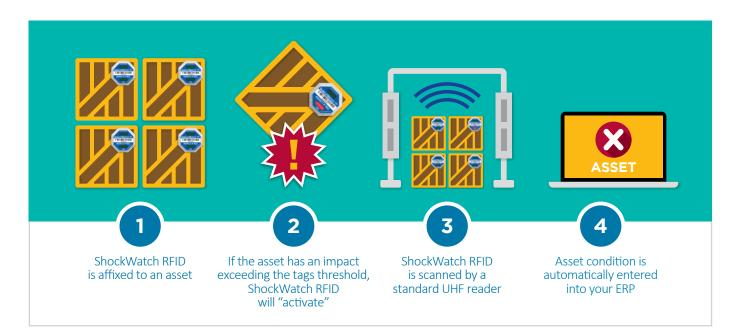
SpotSee's combination of impact monitoring and RFID is a bonus for manufacturers. Not only can cargo handlers and warehouse workers see at a glance which semiconductors or fabrication equipment has experienced potentially damaging impacts exceeding prespecified thresholds (between 5Gs and 75Gs), but that information can be automatically entered to inventory management systems whenever the tags near a passive RFID reader.
