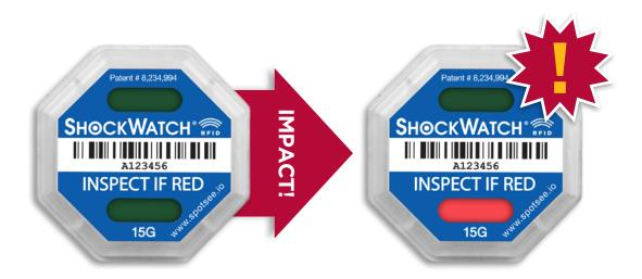
ShockWatch RFID tags turn red when they experienced unsafe impacts, so logistics professionals can spot items that should be inspected at a glance as well as receive an electronic indication. An easy way to do this is simply to affix ShockWatch RFID tags on the cartons being shipped, and then to install passive RFID readers at your facility's loading bay doors and other chokepoints.
