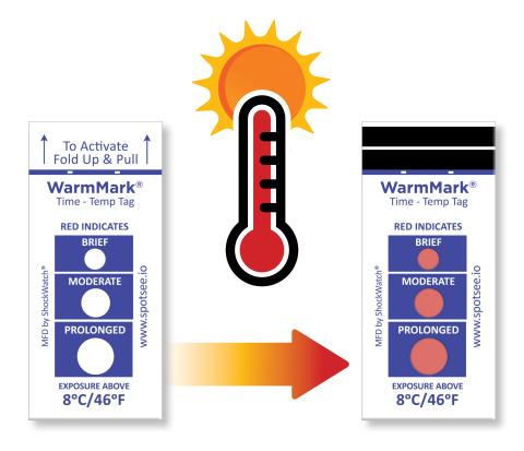
WarmMark is an easy-to-read thermal indicator that turns red when temperature excursions occur. Available in 10 temperature ranges, this temperature indicator features individual dots to signify brief, moderate, or prolonged temperature excursions. Importantly, those terms are defined, and vary based on the temperature threshold of the temperature monitor. For example, "brief" exposure means two hours at 0°C/32°F, but means 30 minutes at 25°C/77°F and above.
